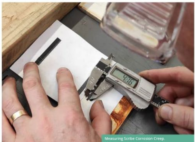
Measuring Scribe Corrosion Creep.
