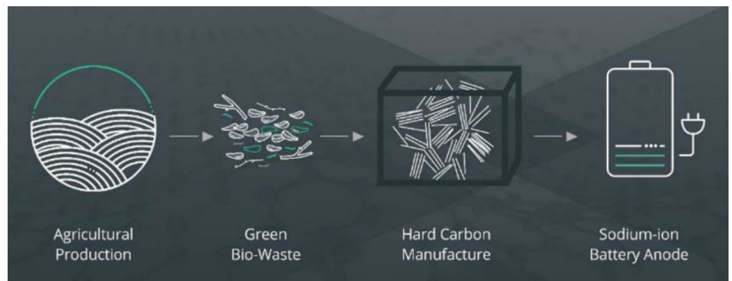
Figure 19: Sodium-ion battery anode manufacturing process
